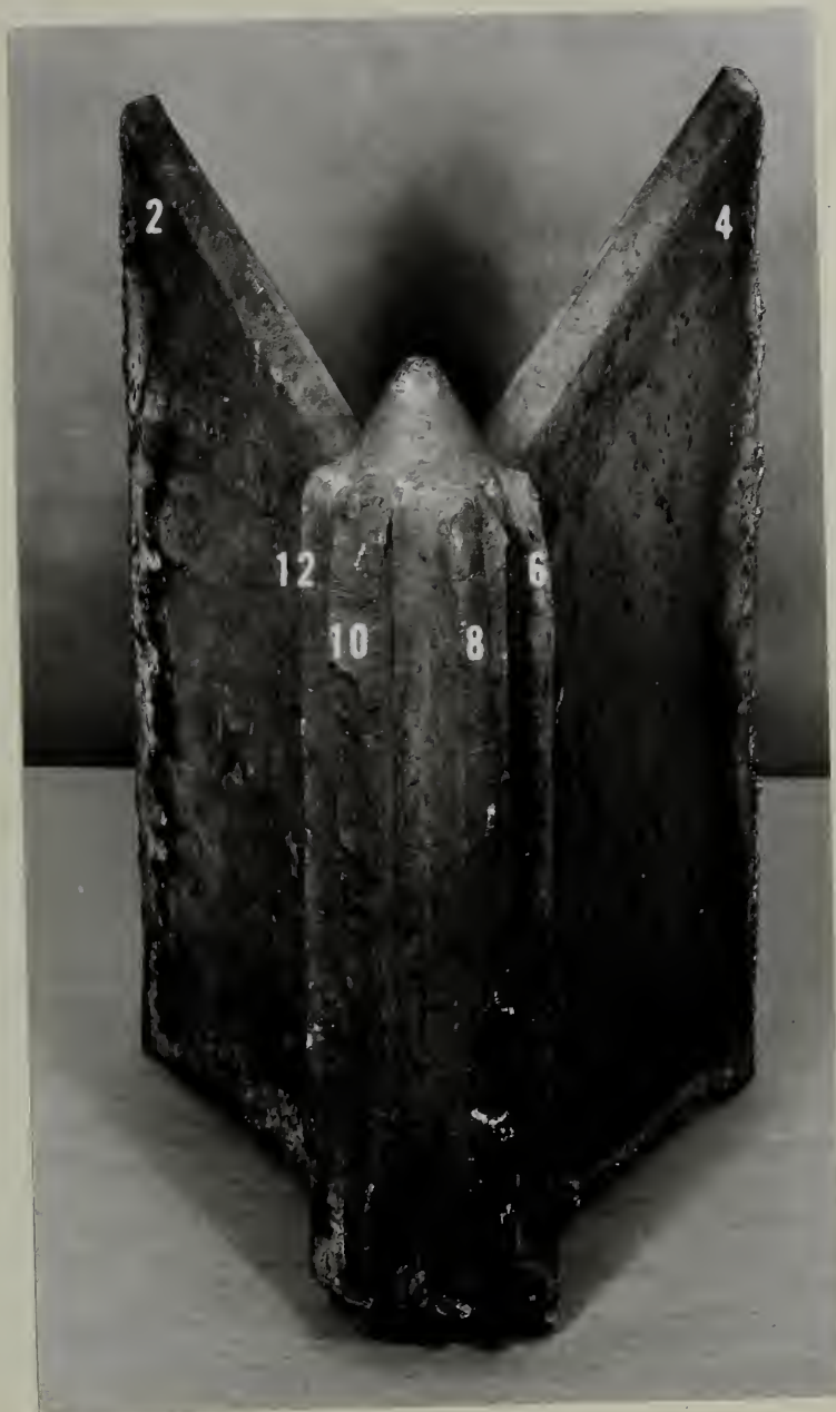
Figure 1. Portion of Howell-Bunger Valve No. 1 as received at NBS. Vane numbers are shown. X 1/4
